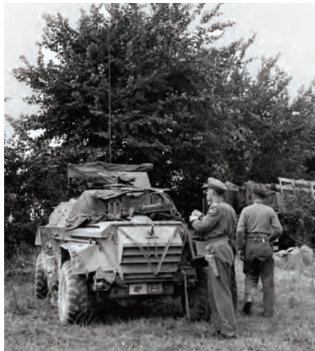
A good rear view of a Humber Scout during the advance into the Falaise pocket. It is noticeable that Humbers often had a lot of stowage on the engine deck. This implies that the crew had confidence in the vehicle's reliability and that they therefore did not need quick access to the engine. KSYM-SAL-19-091
