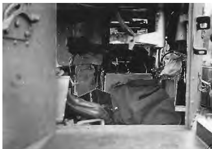
A rare view taken through the rear door of a Crossley where you can just make out the driver's position, along with the lower elements of the turret fittings.
